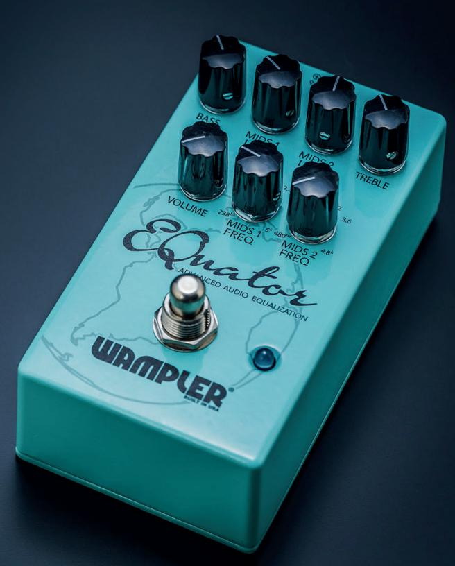
**Bypass** – A relay based true-bypass footswitch that ensures your signal is unaffected when bypassed.
