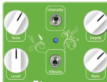
Chorus Detune Depth Intensity Toggle in TOP, Chorus/Vibrato Switch set to DOWN, Tone at 1 o'clock, Depth at between 3 o'clock and fully clockwise, Rate at 9-10 o'clock
