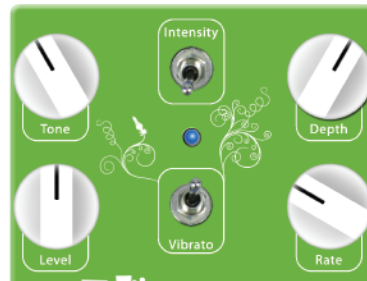
Slow Vibes Depth Intensity Toggle in BOTTOM, Chorus/Vibrato Switch set to UP, Tone at 11 o'clock, Depth at 1 o'clock, Rate at 10 o'clock
