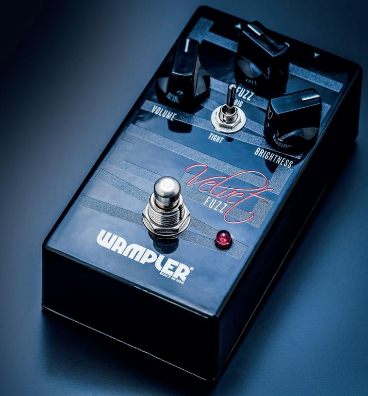
**Bypass Switch** – Simple enough, this relay based soft switch is wired up for true bypass switching to ensure that you don't have anything in the way when you disable the pedal. The LED indicator light will show that when the pedal is activated.
