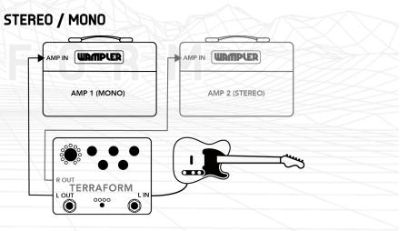
TERRAFORM will understand if you are running in mono - Make sure routing switch is set to **NORMAL**.
